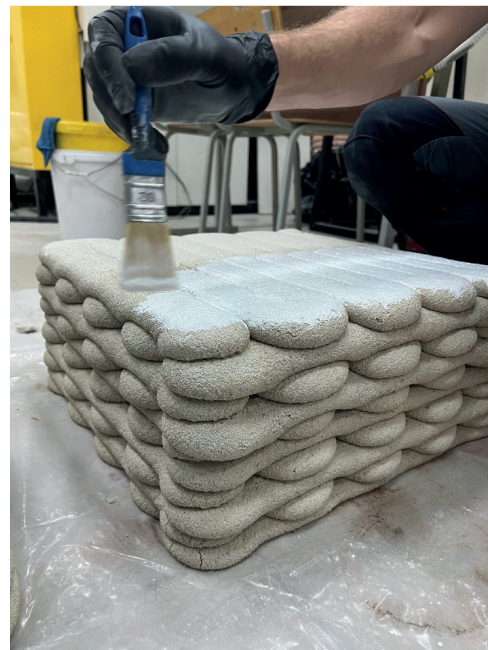
b) concrete contact application process
