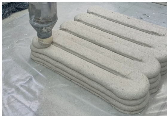
Figure 7. Printing of a parallelepiped-shaped product with layer-by-layer laying of the mixture and different printing heights of the layers
