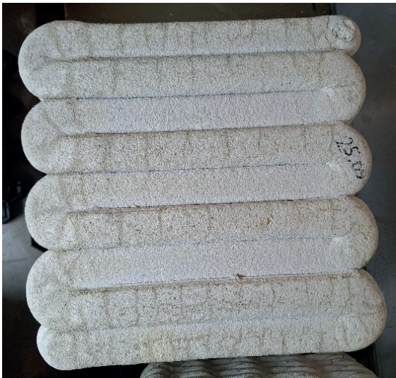
Figure 16. Multiple hairline cracks "spider web" on sample with code 5
