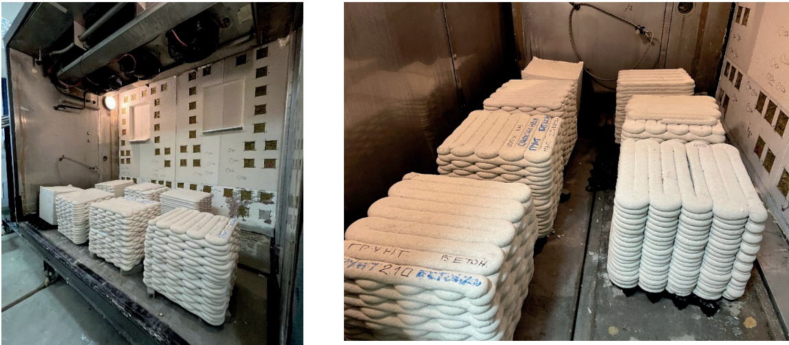
Figure 3. Placing products in a large climate chamber
