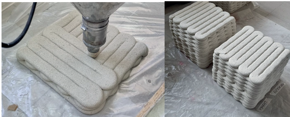
Figure 6. Printing of a parallelepiped-shaped product with layer-by-layer laying of the mixture in perpendicular directions and the appearance of finished products
