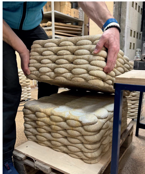
Figure 21. Free separation of the sample by the cold seam modeling zone after 100 cycles of accelerated model aging in a climatic chamber
